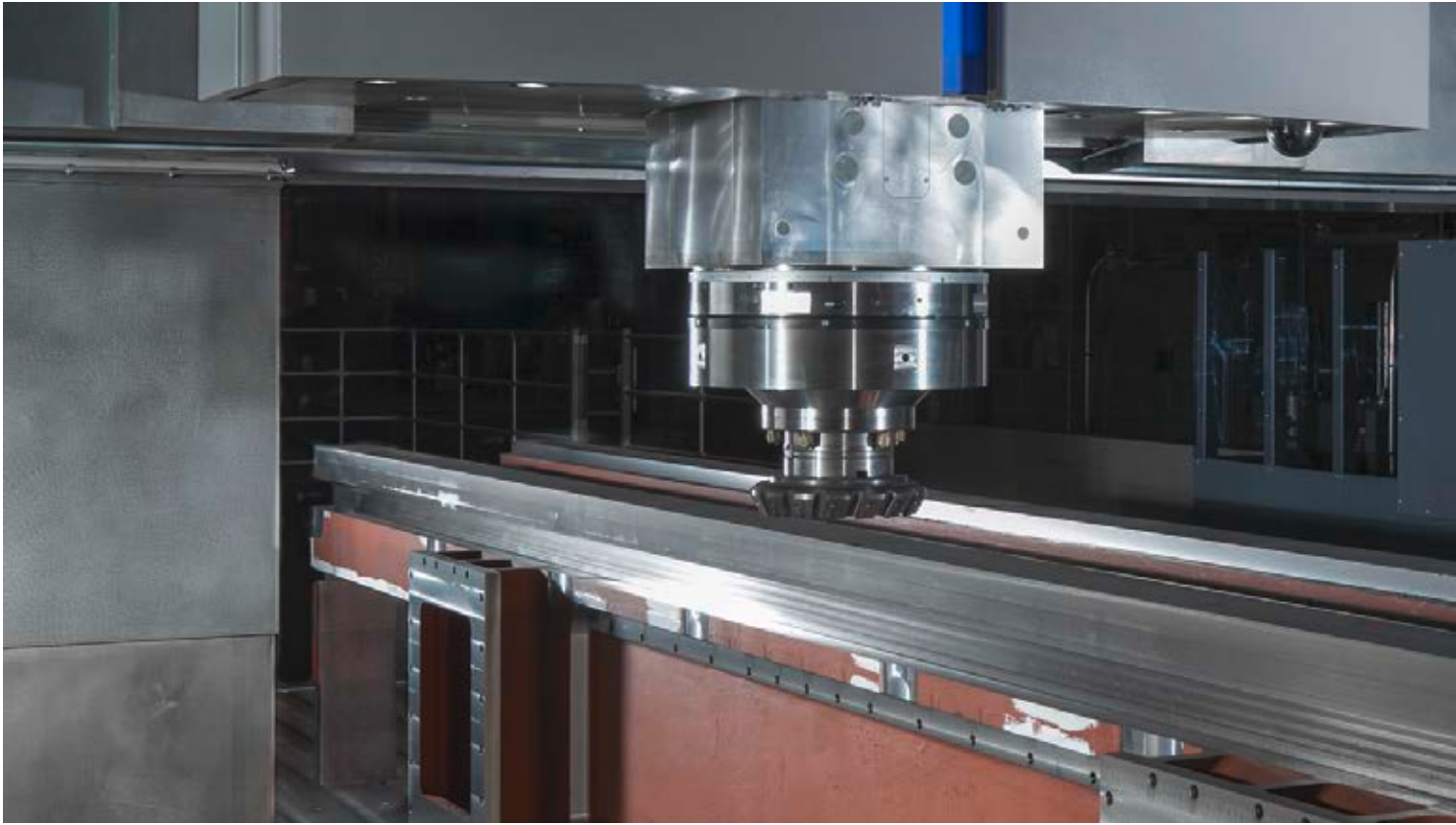
ProfiMill slider with integrated c-axis and milling head
