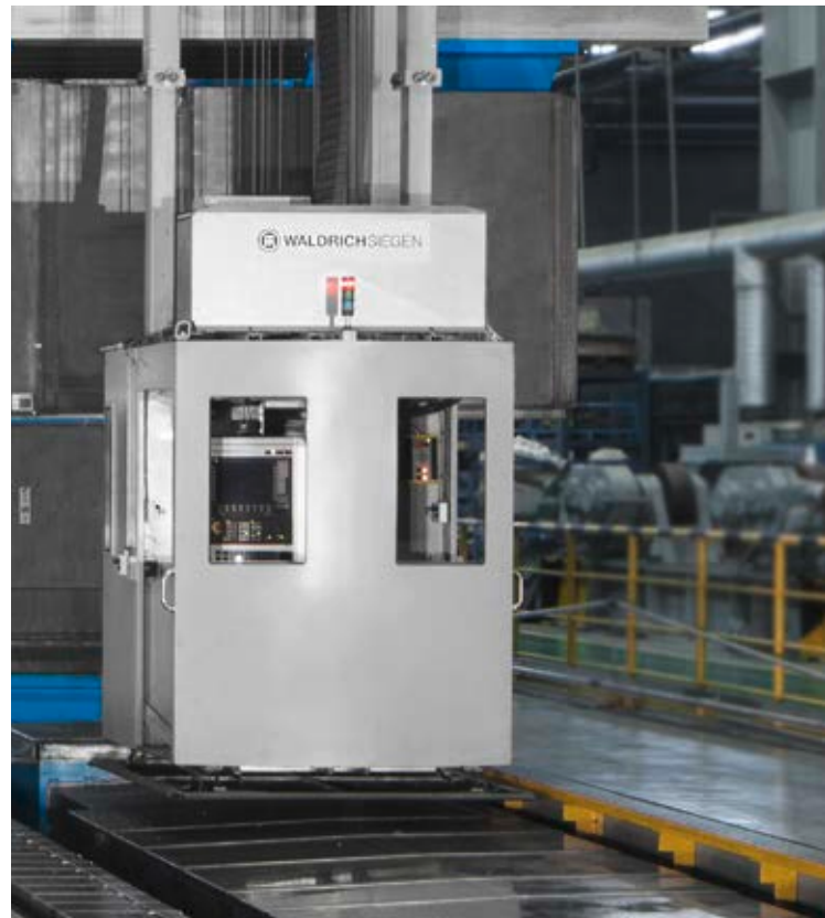
Protected control cabin with view into the working space
