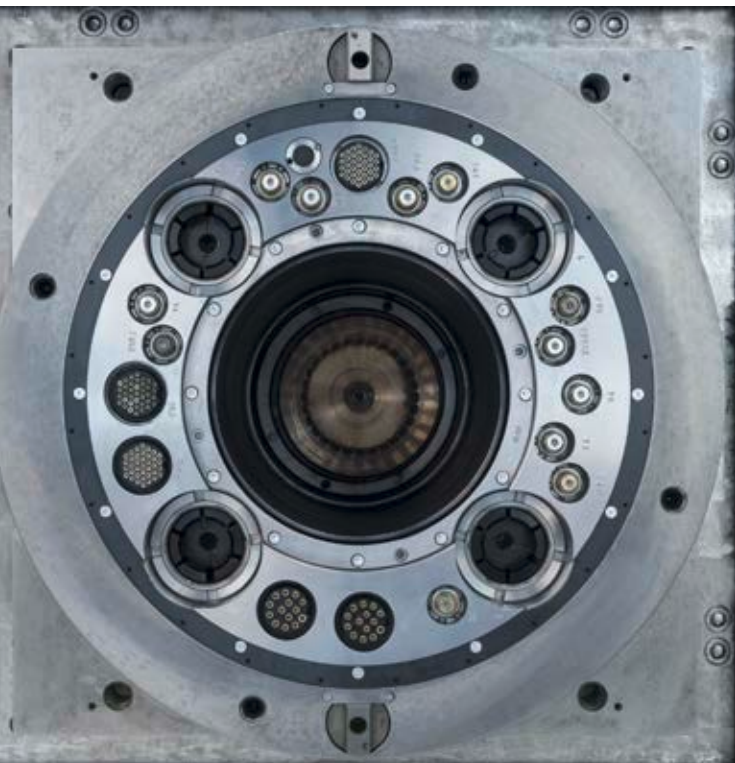
Masterhead interface for different machining units
