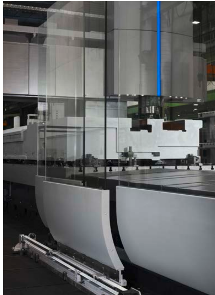
The glass housing provides insights into the work area
